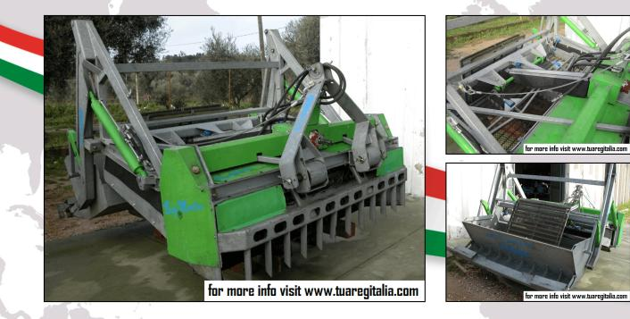
Beach cleaning machine brought by suitable tractors (80-90 HP) with four-wheel drive, equipped with hydraulic lift. It works for a width of 190 cm. The work capacity indicated by the manufacturer is 7000-15000 sqm./h and over, depending on the quality of the sand (wet, damp, dry) and the condition of the beach. The working depth, adjustable by a hydraulic lift of the tractor, varies from 0 to 20 cm.
