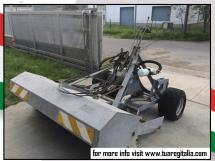
Beach cleaning machine brought by suitable tractors (90-120 HP) with four-wheel drive, equipped with hydraulic lift. It works for a width of 200 cm. The work capacity indicated by the manufacturer is from 15,000-25000 sqm./h. The working depth varies from 0 to 15 cm.
