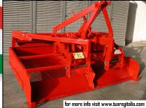
Beach cleaner made by the historic Collina company in Pescara. We permuted and arranged in all its parts, including the gearbox, eccentric shaft and bearings. The rear roller has also been totally regenerated, as well as other components. Working width is of about two meters.
