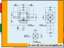
Gearboxes by Bondioli & Pavesi brand. As shown in the photos it is in cast iron and is new. Common entrance grooved connection for universal joint and 'double' outlet with smooth shaft diameter 22 mm and keyway size 6x6x30 mm. Ratio 1: 1.35, with a power of 20 hp. This box is sold in the shop for about 350 euros.
