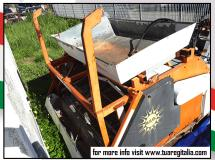
The beach cleaner works mechanically taking the moving power directly from the PTO (power take-off) of the tractor to which it is connected through the 3 point attachment of the lift system. It is also able to regulate the working depth from 0 up to 15 cm per 160 cm of width. The sand and the debris are charged by a set of nylon scrapers activated by a chains system. They charge the sand and the debris on a grid frame which is as wide as the machine is and 60cm tall and which works as a sifter.
