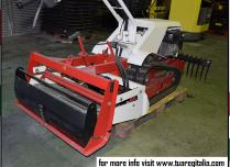
The S90 beach cleaner is a self-propelled track-driven machine, ideal for cleaning sandy areas. The speed of the machine and the operation of the sieve they are independent of one another through a HYDROSTATIC system that makes it unique in the sector unlike traditional mechanical transmission machines.
